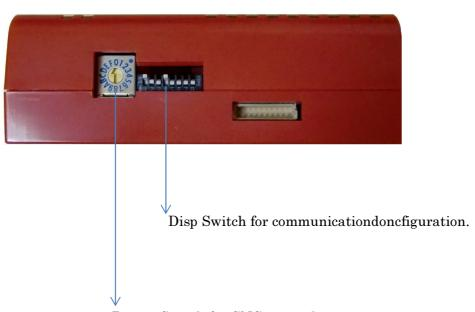
Rotary Switch for CNC type selection.
